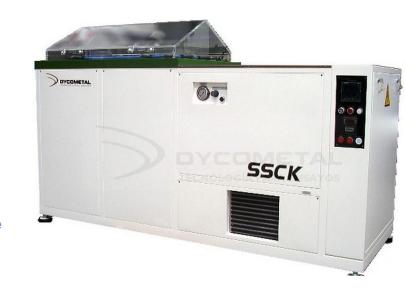
After making the test based on the Japanese Cyclical Corrosion Test (C.C.T.), most of the automobile's manufacturers have checked that with this Chamber they get better results than the ones of the Salt Spray Chamber because of its faster corrosion velocity.
